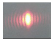
The laser beam center is positioned 1/2 inch from the bottom of the level. This means that a half inch needs to be subtracted from the center spot of the laser dot to reference the actual bottom of the level.
